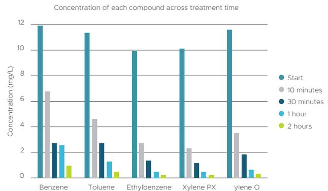
The trial showed that BTEX compounds can be oxidised down to low levels. Trials achieved over 96% removal on average (average of the 5 compounds). Dependant on individual concentration targets, treatment can be prolonged, or parameters adjusted, to reach levels in line with strict regulation.
