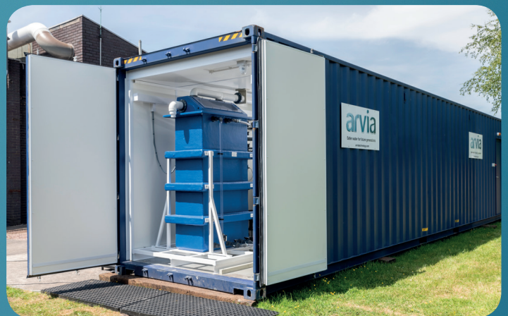
Full scale Nyex containerised system
